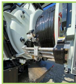
Tank Door, Hose Reel & Hose
